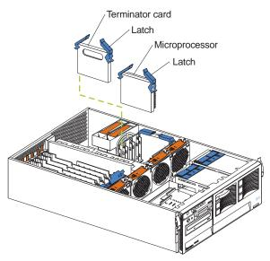
To install an additional microprocessor:
